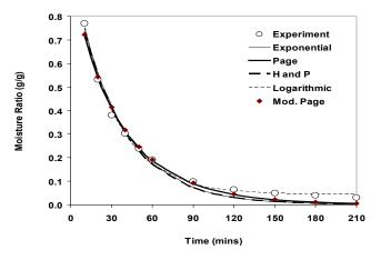
Figure 6. Experimental and predicted moisture ratio for SOSAT C88 at 70°C
