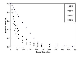
Figure 3. Moisture ratio for SOSAT C88 millet
