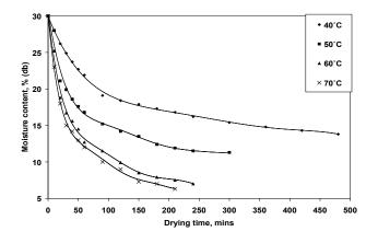
Figure 2. Drying curve for EX-BORNO millet
