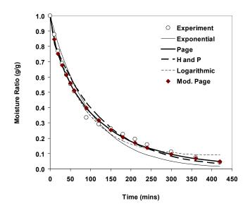
Figure 7. Experimental and predicted moisture ratio for EX-BORNO at 40°C
